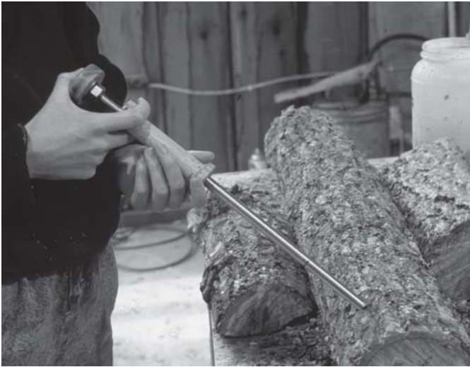
Figure 5. Sawdust spawn inoculator.
