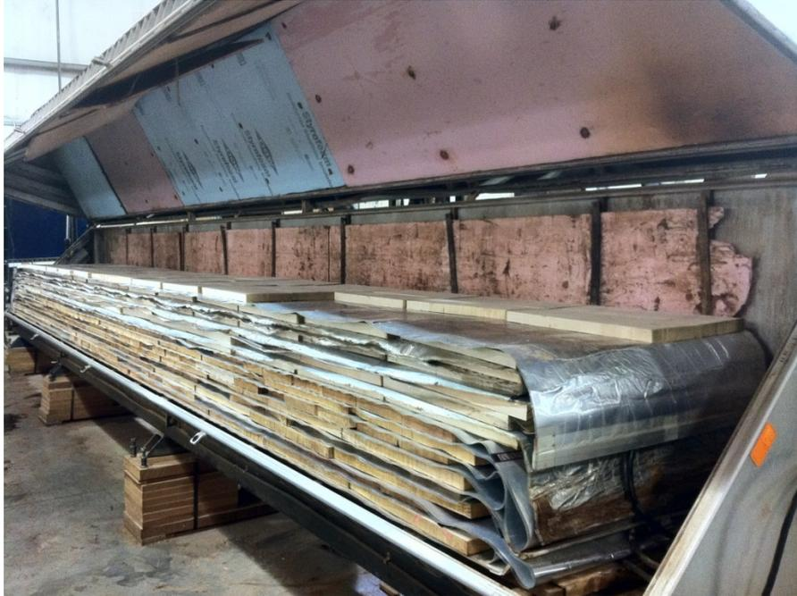
**Figure 2.** This clamshell-like vacuum kiln is used to dry high-value hardwood blanks for a guitar factory. The silvery pieces of fabric are used to heat the wood.
