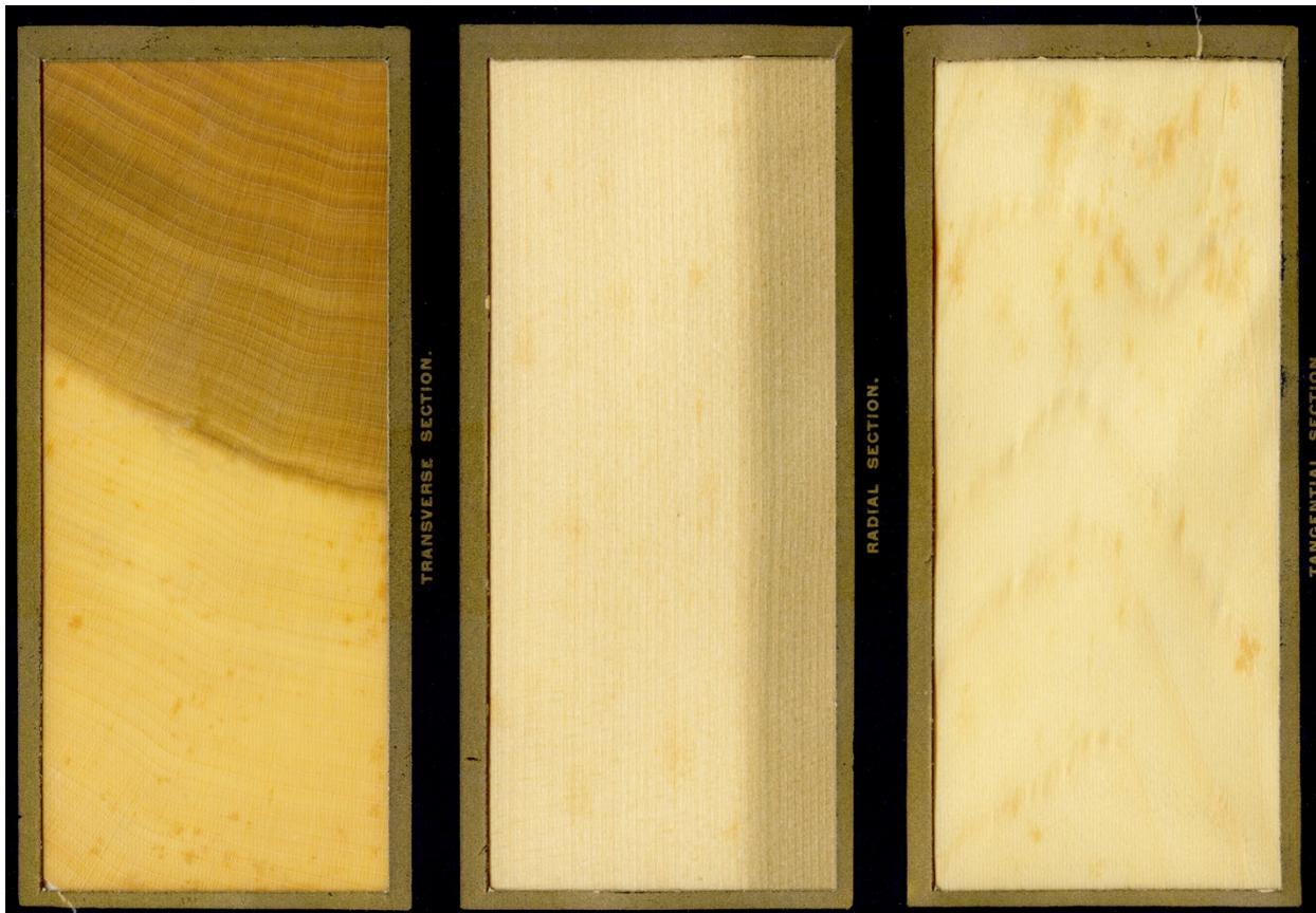
**Figure 13.** This is a photograph of a cross section (marked transverse section), a radial section, and a tangential section of yellow-poplar, a diffuse porous species. Earlywood pores are not obvious at this magnification, unlike in ring porous species.
