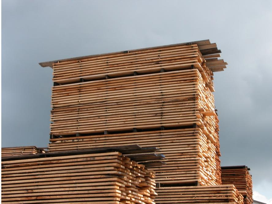
**Figure 33.** This lumber is well stacked and the yard manager has added stack covers (made of weighted-down boards in this case) above the top layer of lumber to protect the lumber. Note the stickers used to keep the stack covers away from the top layer.
