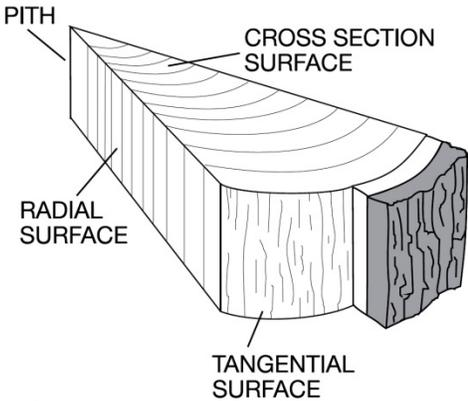
**Figure 11, repeated.** This sketch labels the three wood faces on a wedge of wood. Ray sides will look like ribbons on radial faces, and the ray ends will look like short lines on tangential faces. Rays will also be visible on the cross-section extending from the direction of the pith towards the bark, in the radial direction.
