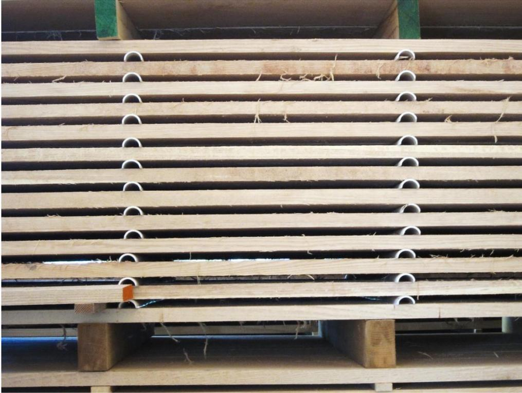
**Figure 37.** *Cut 1-1/2" PVC pipe can be used to make light-duty stickers with good air flow characteristics. The stickers should have been better aligned with the bolsters here.*
