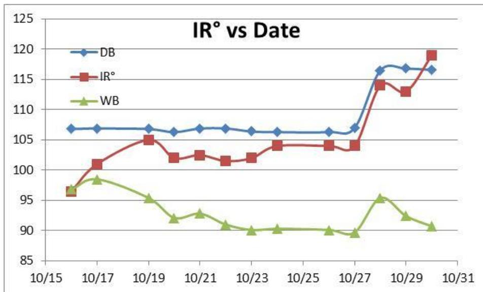
**Figure 17.** Data from a commercial DH kiln run with hickory sapwood. The surface temperature readings taken with a handheld infrared thermometer approached the dry bulb temperature on October 24<sup>th</sup>. DB= dry bulb temperature (°F), WB = wet bulb temperature (°F), and IR° = the infrared thermometer reading (°F). The IR thermometer readings aren’t as precise as the kiln temperature readings, and so they appear to vary more than the kiln temperature readings.
