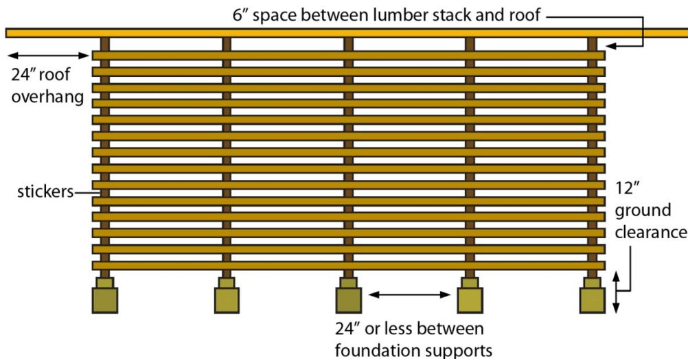
**Figure 40.** Side view of a well-stacked pile of hardwood lumber.
