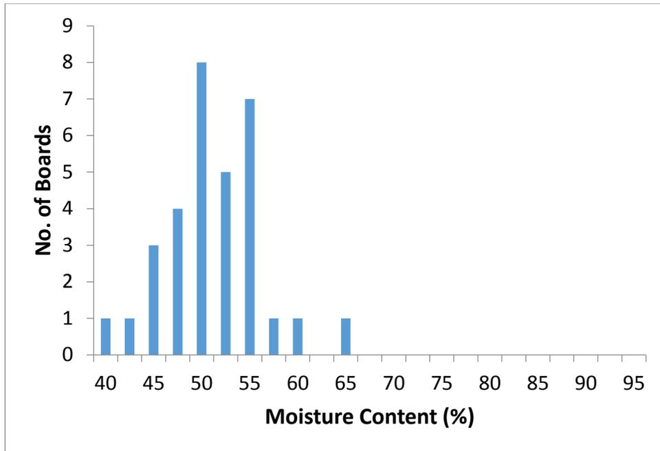
**Figure 21.** This is a simulated distribution of the moisture contents of 38 green hickory sapwood boards. The overall average moisture content is 51%.
