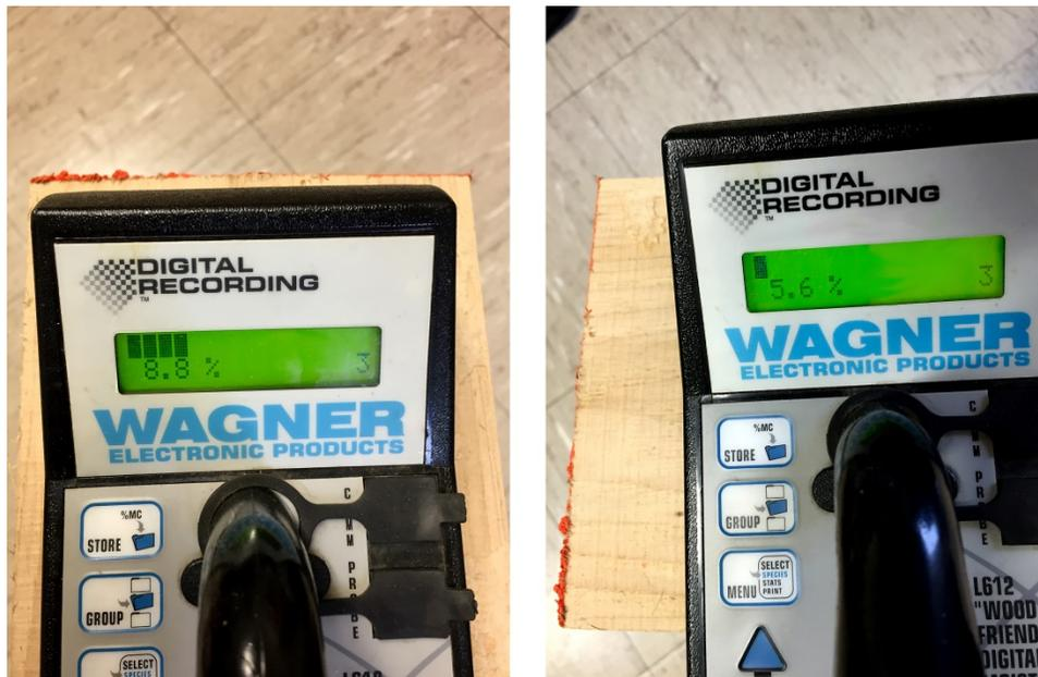
**Figure 46.** Different readings with a dielectric moisture meter on the same (cupped) board. The meter is parallel to the grain in the left-hand photo and turned at 90° to the grain in the right-hand photograph.
