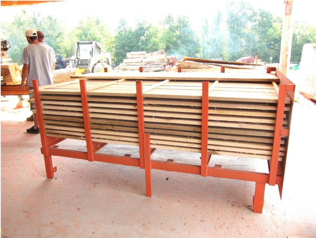
**Figure 31.** This is an example of a steel U-Channel stacking jig for 8' lumber used at a small Kentucky sawmill. Boards and stickers are placed by hand.
