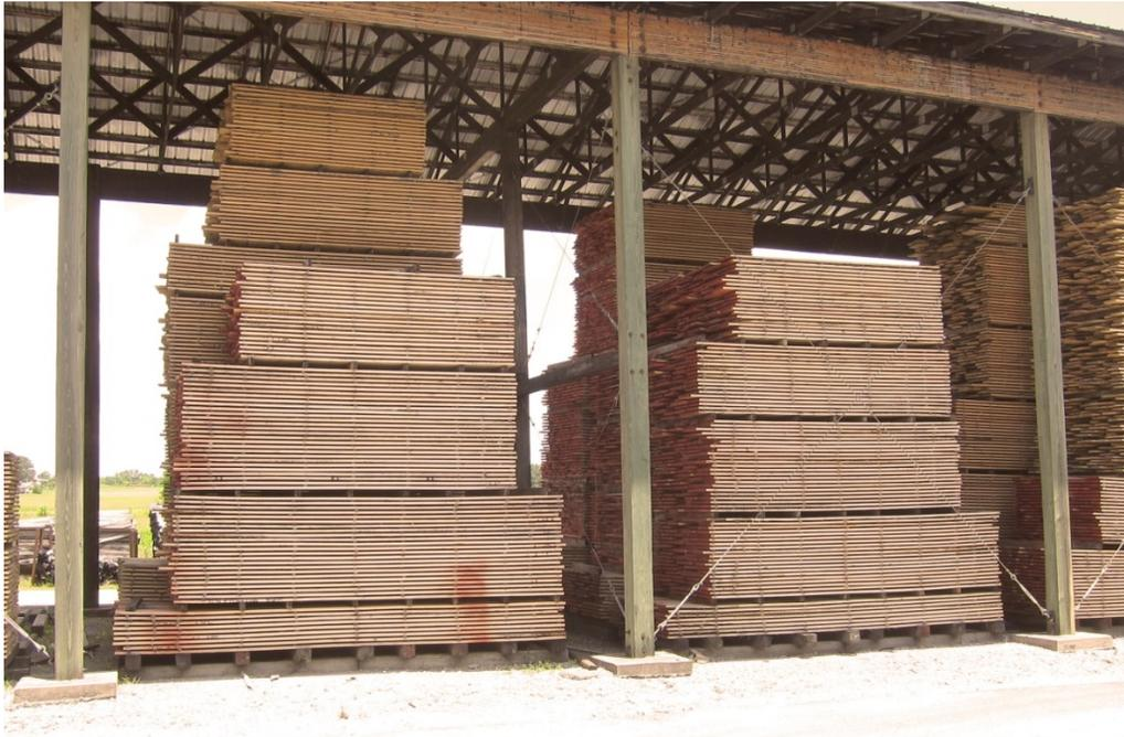
**Figure 32.** This is a good example of how to stack air-drying lumber. The piles are supported by doubled bolsters and there is no vegetation. The fork truck operator placed the piles directly atop the bolsters and the stickers are nicely aligned with the bolsters and the packs above. At this location the lumber is drying under a shed roof, but stack covers could be used as well.
