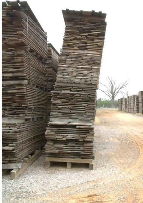
**Figure 45.** Don't position your stacks like this! In spite of the obvious problem with this pile of lumber, this yard has tried to do things right. The piles have stack covers, the yard looks well-drained and free of vegetation, and the lumber is placed on double bunks to raise it off the ground.
