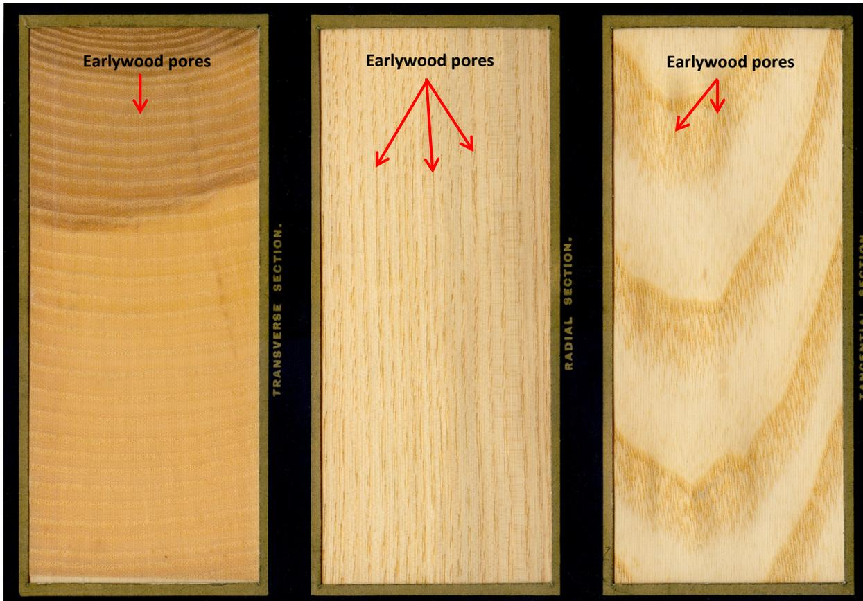
**Figure 12.** This is a photograph of a cross section (marked transverse section), a radial section, and a tangential section of white ash, a ring porous species. Some of the earlywood pores are marked.
