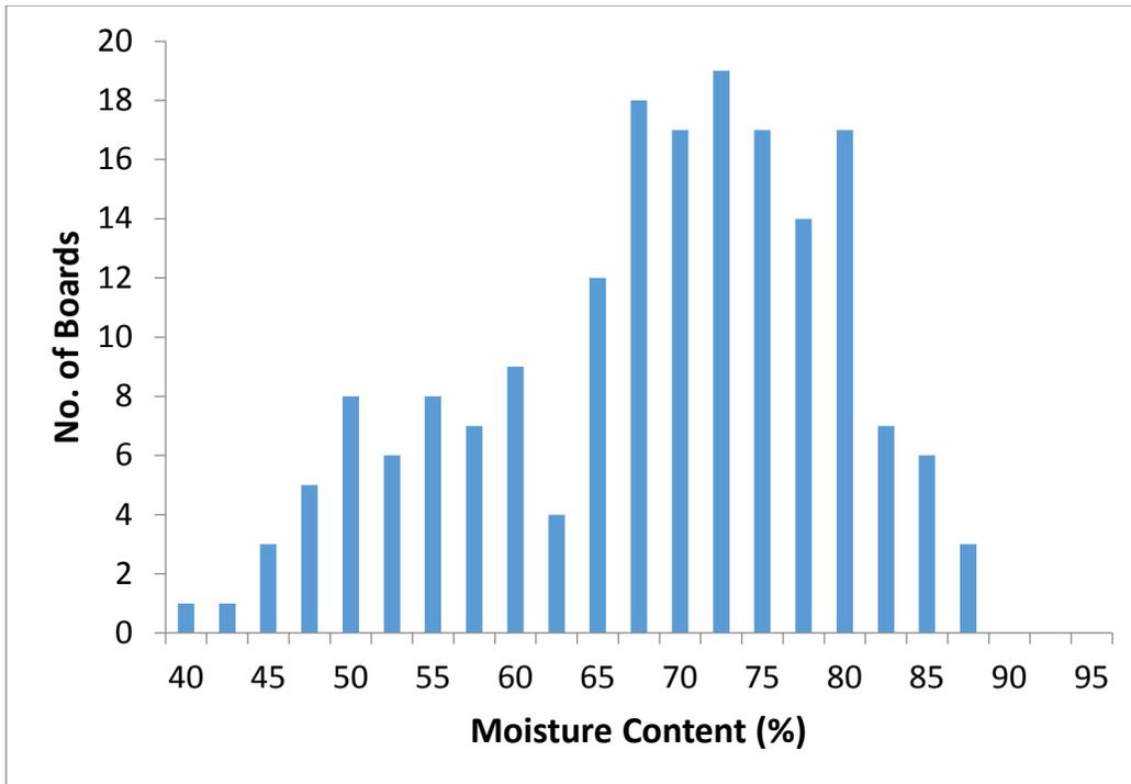
**Figure 22.** This graph combines the simulated distribution of the moisture contents of the previous 150 green hickory heartwood boards (70% average MC) and the 38 green hickory sapwood boards (51% average MC). The overall average MC for heartwood and sapwood combined in this example is 67%.
