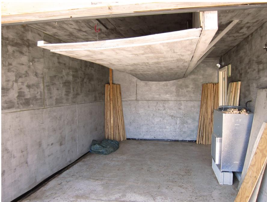
**Figure 4.** In this DH kiln the compressor unit is to the right. The hinged piece of plywood near the ceiling is a baffle that drops to direct circulating air through the stacks of lumber. There is a small powered vent at the rear.
