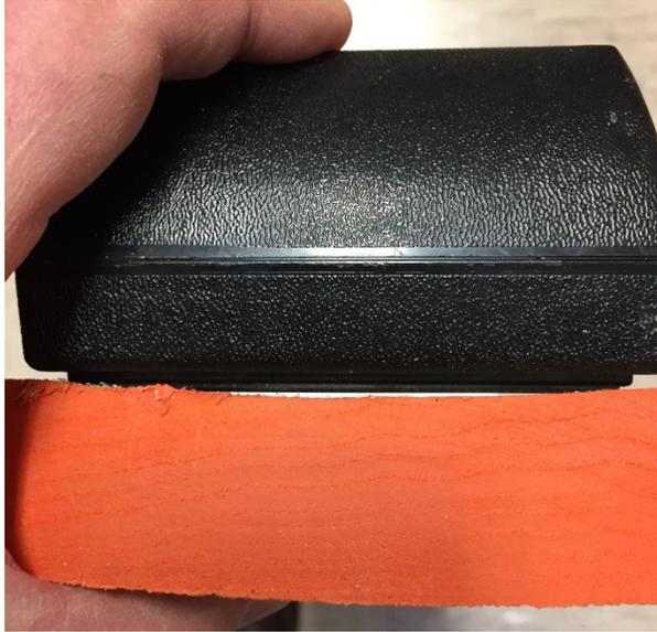
**Figure 48.** Dielectric moisture meter oriented parallel to the grain on the same board as in the previous figure. Poor contact between the board and the meter electrode plate will prevent accurate moisture readings.
