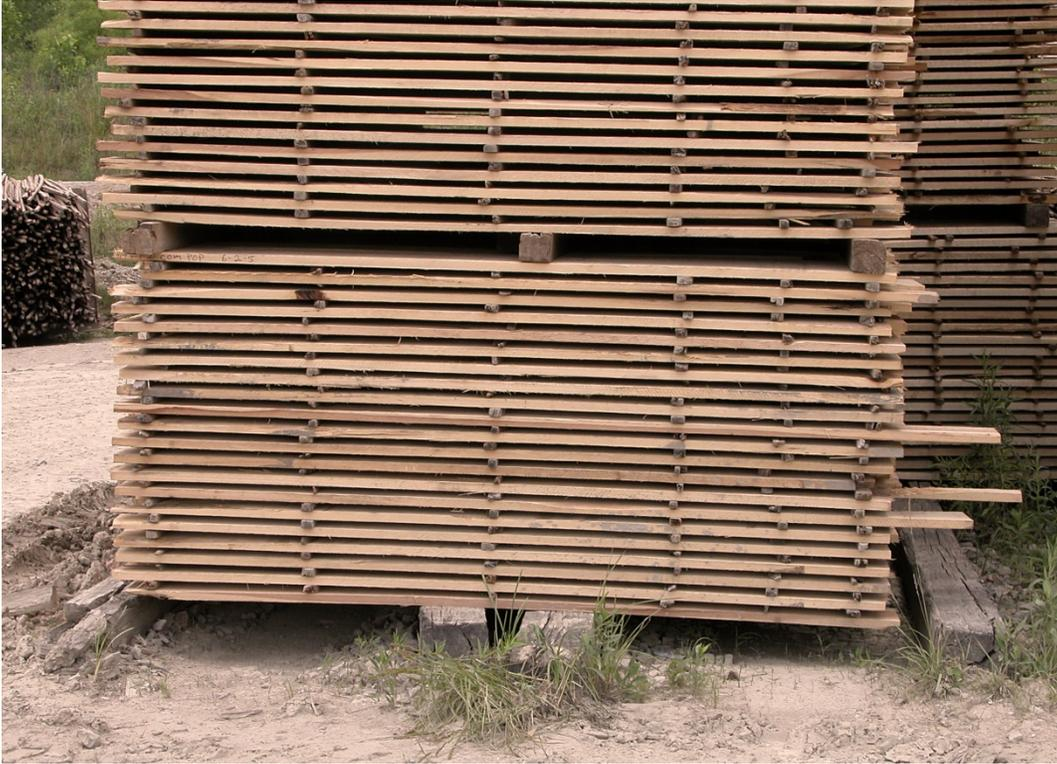
**Figure 44.** *There are several problems with this stack of lumber. The stack isn't high enough off the ground, the lumber isn't supported properly all across the load, the yard is weedy, the sticker alignment could be improved and the lumber isn't all a uniform length.*
