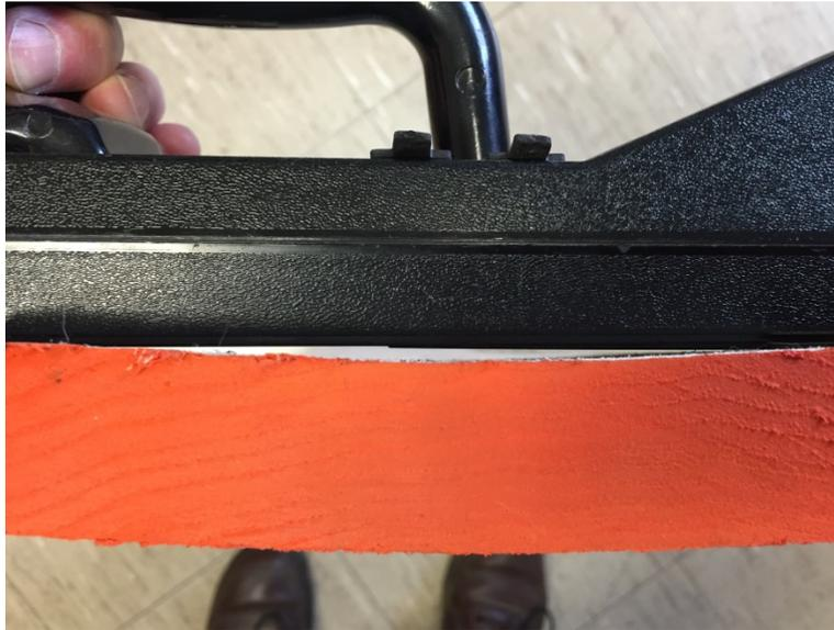
**Figure 47.** Dielectric moisture meters cannot make an accurate reading if the electrode plate can't make full contact because the lumber is cupped. In this photo the meter is perpendicular to the grain.
