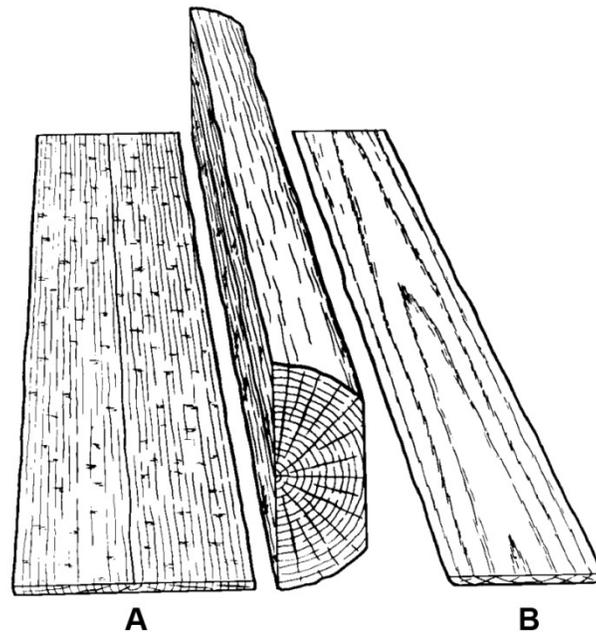
**Figure 14.** This figure shows (A) a quartersawn board and (B) a flatsawn board. In quartersawn boards the rays are parallel to the wide dimension, and in flatsawn boards the rays run perpendicular to the broad surfaces.
