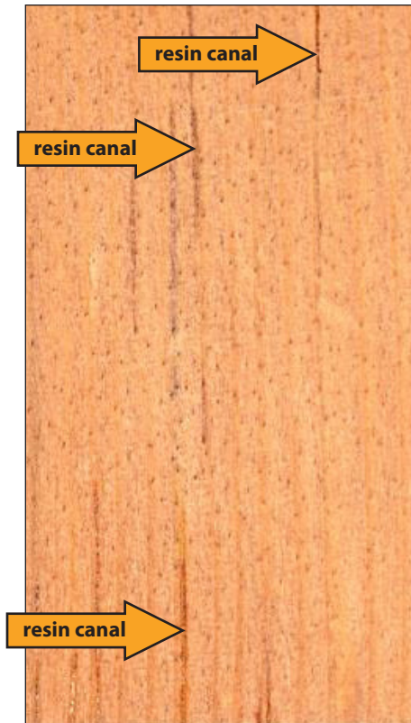
Figure 5-4. The vertically oriented brown streaks in this sample of sugar pine ( P. lambertiana ) are longitudinal resin canals and the small brownish specks are the ends of the resin canals in fusiform rays. (Not every resin canal in the photograph is labeled.)
