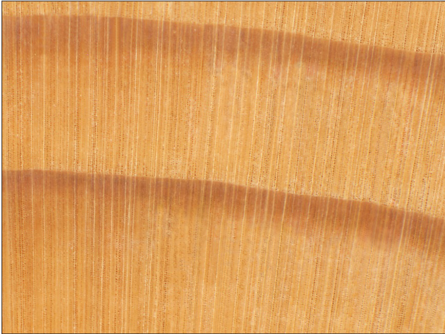
Figure 5-1. This micrograph of a single growth ring of western redcedar ( Thuja occidentalis ) shows earlywood tracheids, latewood tracheids, and rays.
