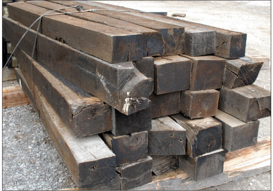
Figure 6. This is a bundle of culled crossties at a tie plant. There's more than one kind of problem shown here, but several ties were apparently culled because they were bucked too short for felling cuts to be removed by the plant's cut-off saws.
