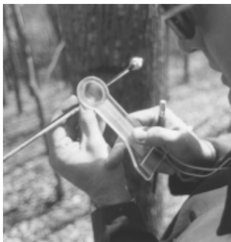
A forester examines a wood core extracted from a tree to determine its age and growth rate.
