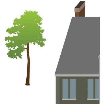
Prune trees from the ground to 10 feet up and trim any overhanging branches to prevent fire from transferring to your roof.
